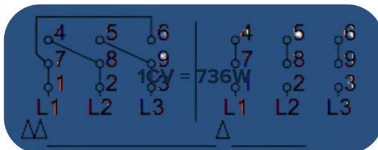
WIRING DIAGRAM ON MOTOR BOARD
